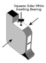
A nice idea is to use a Pony Clamp to squeeze sides of cartridge, see our Accessories Page. It provides the squeeze and keeps cartridge upright in the process.
